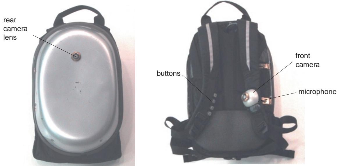
Figure 3: The Data Collection Wearable Schematic
