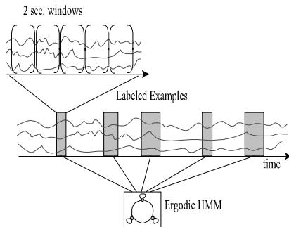
These features,  $\{x_t\}$ , were modeled by ergodic Hidden Markov Models (HMM). To train the HMMs, each example of a location was divided into 2 sec. windows (or equivalently,  $N = 10$  feature vectors at 5Hz) of features. These windows of features were gathered into one set and used to train a class HMM (with Expectation-Maximization). By design, the class HMMs, when trained
