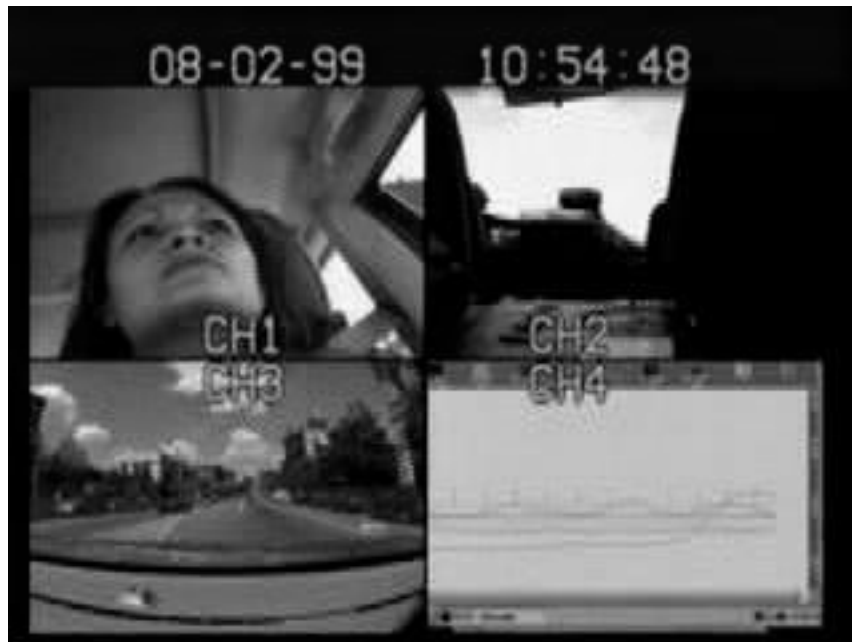
Figure 5-2: A sample frame from the video collected during the experiment. Views of the driver facial expression (upper left), body movement (upper right) and road conditions (lower left) are combined with the microphone input and a visual record of the physiological signals (lower right)
