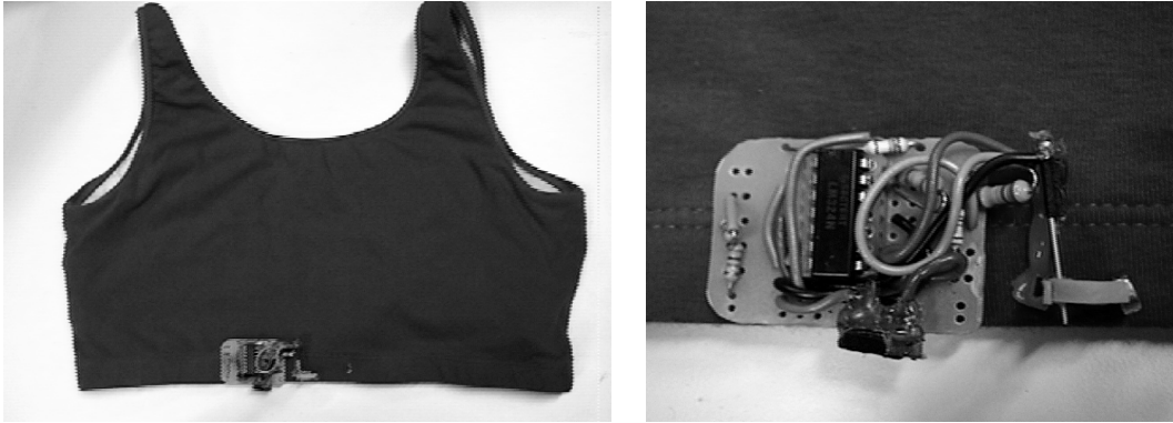
Figure 4-8: A prototype for respiration sensing through chest cavity expansion using a Hall Effect sensor. The left image shows the sensor in the location where it could be embedded into a sports bra. A close up of the sensor in the right image shows the analog components and the constrained magnets. This image does not show the attached ADX board.
