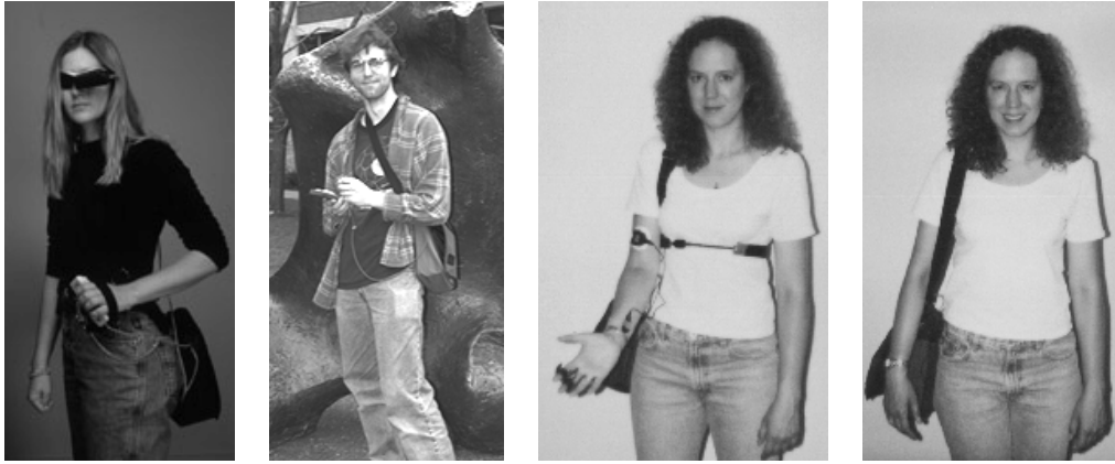
Figure 4-2: To make the wearable monitoring system less noticeable, a PalmPilot interface was developed to replace the head-mounted-display and chordic keyboard. The physiological sensors can be worn underneath clothing.
