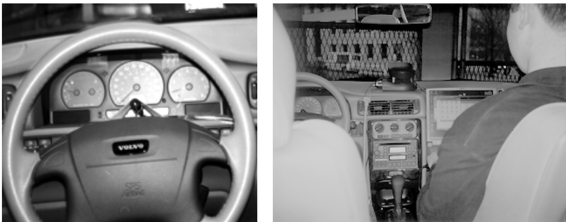
Figure 5-3: A small camera is placed on the steering column to capture facial expression while driving. A second camera monitors driver body motion and allows the observer to mark events using index cards.
