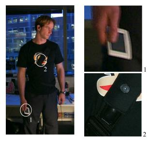
Table 1 The labeling wearable: (1) the touch sensitivepad for Unistroke input, (2) sensor package containingpinhole CCD and boundary microphone.
