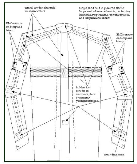
Figure 1. Placement and integration of sensors into the jacket.
