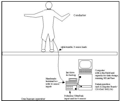
Figure 2. Hardware Architecture for the Conductor's Jacket.
