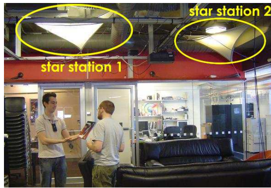
Figure 4. Follow the Star : An environment with two star stations. The color light bulbs illuminate when the target is underneath: green when the target is available and red when they are not.
