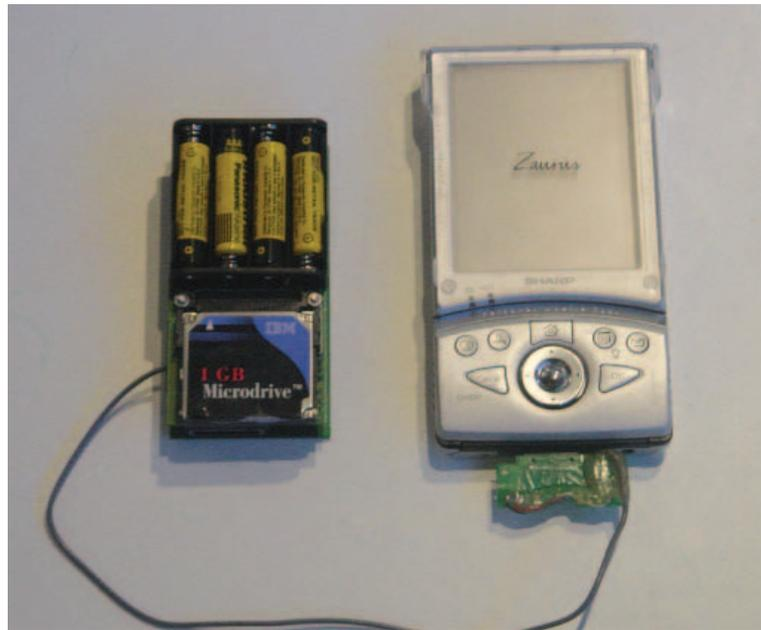
**Figure 1. MITHril system. Plugging the biosensor hub into a cell phone or wireless PDA provides a system that offers input, output, and general computation functions and can support a wide range of physiological measurements.**
