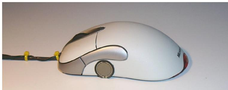
sitive resistor, we continued to develop the idea of treating the mouse less like an interface and more like a sensor. To this end, we made a Squeezemouse which used 144 small force sensitive resistors to cover the surface of the mouse. During the development of this mouse, we discovered that the Force Sensitive Resistors were not sensitive enough to transduce the small load placed on them by the hand resting on the mouse.
