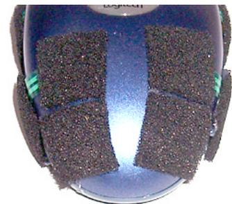
Figure 51: Pressuremouse tactile sensors.
