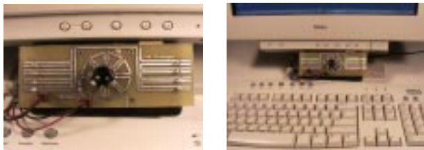
Figure 2. Camera to track pupils, placed under the monitor
