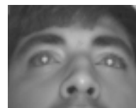
De-interlaced sampled image, when the on-axis LEDs are on
