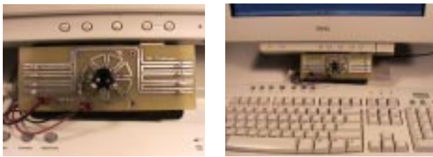
Figure 3. – Camera to track pupils, placed under monitor.
