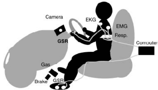
Figure 1: Above: a sample frame from the video collected during the experiment showing driver facial expression and road conditions synchronized to the real-time physiological responses. Below: a diagram showing sensor placement. GSR sensors are placed on both the hand and the foot.
