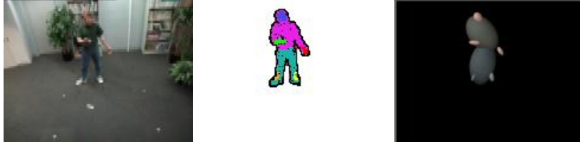
Figure 4: Analysis of a user in the interactive space. Frame ( left ) is the video input (n.b. color image possibly shown here in greyscale for printing purposes), frame ( center ) shows the segmentation of the user into blobs, and frame ( right ) shows a 3-D model reconstructed from blob statistics alone (with contour shape ignored).
