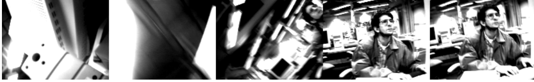
Figure 8: StartleCam creates a composite image from a buffer of digital images recently captured by the wearer's camera. In this sequence, the wearer was surprised by a question from a friend. The sequence shows images captured as the wearer turned to address her friend.
