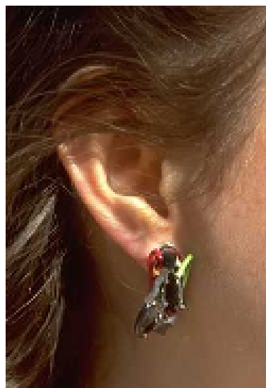
Figure 10: Analog BVP sensor in earring attachment for use with infrared or PAN A/D processing units (Photograph by Frank Dabek).
