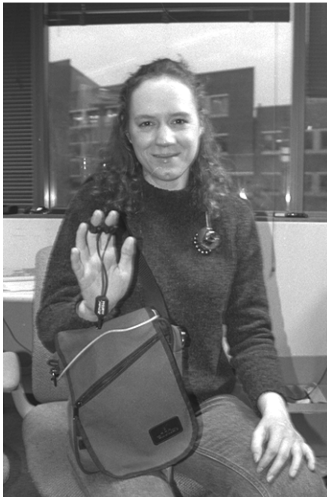
Figure 1: The StartleCam system, consisting of a wearable computer (lower left), electrodes to measure skin conductance (center left) and the digital camera (center right). Photo courtesy of Frank Dabek
