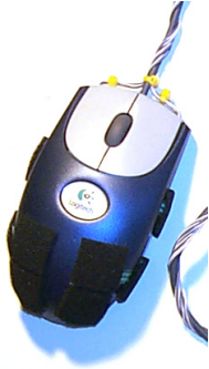
Figure 1: PressureMouse: four foam sensors at the back of the mouse and two on each side.
