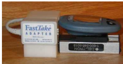
FIGURE 5. The challenge with using the FastTake meter was that the same slot on the meter had to be used both for glucose strips while measuring, and for the adapter when transmitting data. Shown is the final design by Meza to solve this problem.
