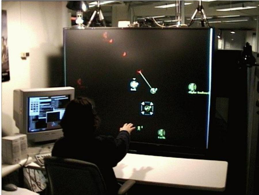
Figure 3.2: Netrek Collective Interface: the user uses a deictic gesture to select  $F0$ . Cameras on top of the display track the user's movements and a head-mounted microphone is used for speech recognition.
