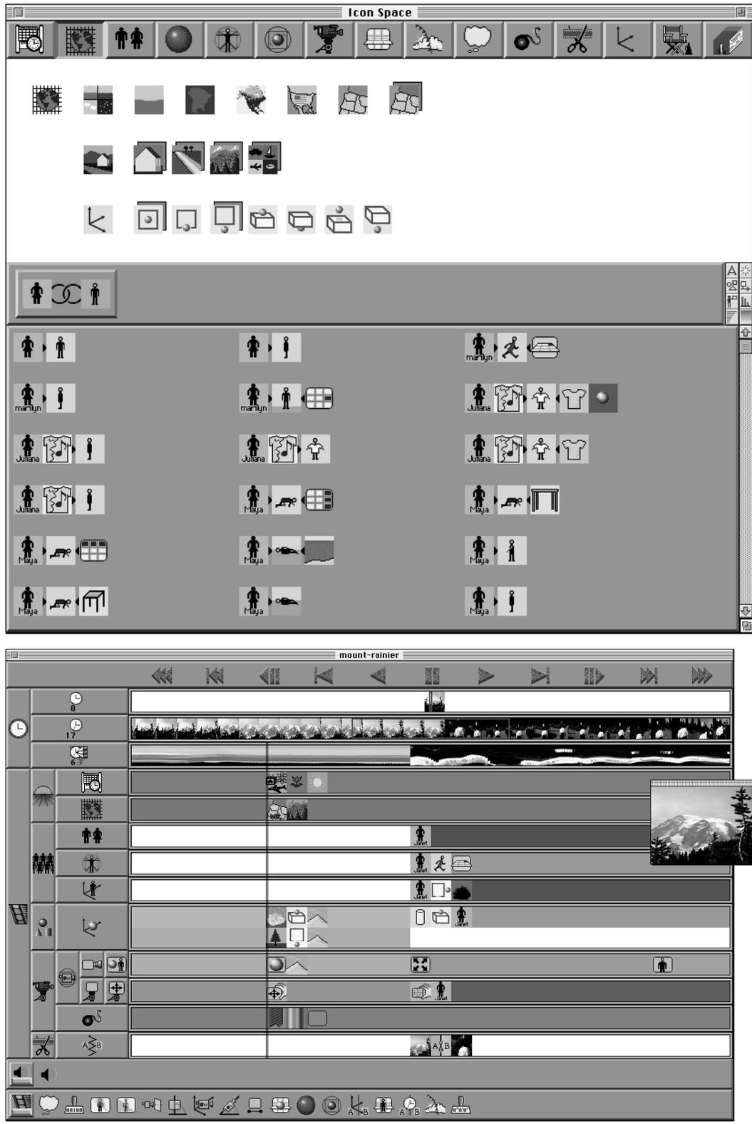
Figure 6: The upper image shows the icon palette used by MEDIA STREAMS for annotation; this illustrates some of the icon language's spatial relationships. The bottom image shows how the icons are used to produce a layered annotation of a video stream.
