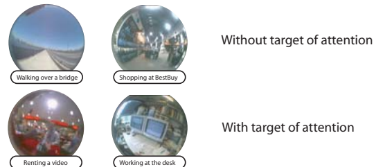
Figure 0-1: Two beneficial side-effect of the fish-eye lens. Objects receiving the wearer's visual attention cover more pixels. The wide-angle capture enables a complete but low resolution sampling of the periphery.
