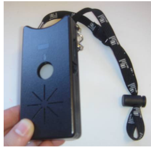
Figure 1. The sociometric badge, an example of a sensor-based system that detects individual and social behavior in real-time allowing real-time feedback.
