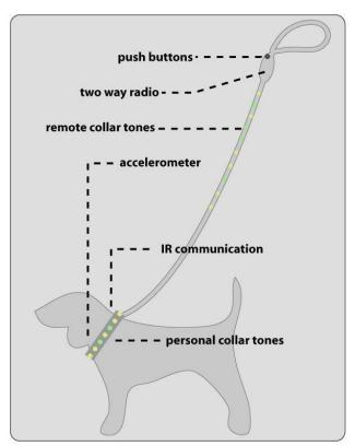
Figure 1 Components of the SNIF System
