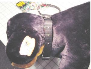
Figure 3: Top picture shows the collar with its modified UbER-Badge. Lower picture show how the collar fits on the stuffed dog.
