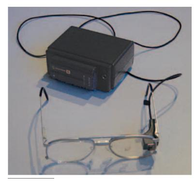
Figure 2. Memory glasses. A wearable, proactive, contextaware memory aid, the memory glasses system combines the MIThril platform with wearable sensors to provide a device that functions like a human assistant, storing reminder requests and delivering them under appropriate circumstances.
