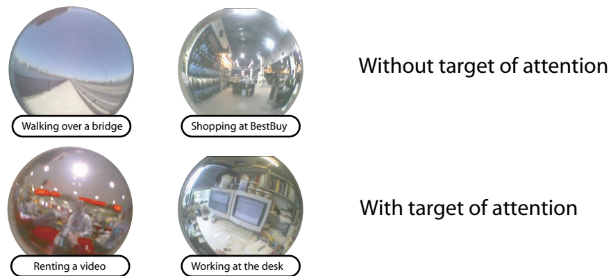
Figure 5-2: Two beneficial side-effect of the fish-eye lens. Objects receiving the wearer's visual attention cover more pixels. The wide-angle capture enables a complete but low resolution sampling of the periphery.
