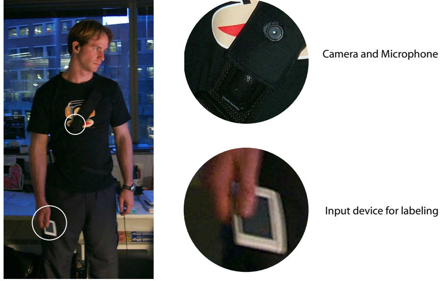
Figure 3-6: The wearable used in the experiments on situation dynamics and transitions. It is a primitive data collection system consisting of a pinhole camera mounted on a shoulder strap and a handheld mouse pad for data entry and labeling.
