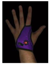
Figure 21: Jocelyn Scheirer's galvactivator communicates skin conductivity through a LED and a jack which analog data can be acquired through.
