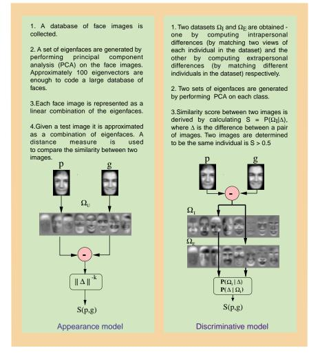
Figure 3: Face Recognition using Eigenfaces
